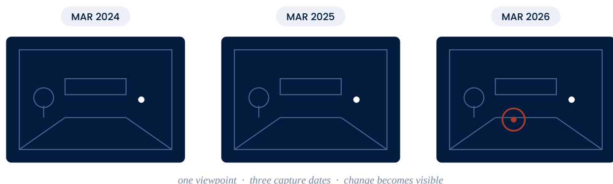
Figure 4. Same-viewpoint re-capture: one plant-room viewpoint across three capture dates. Condition change stops being a matter of recollection and becomes a comparison of dated images.
